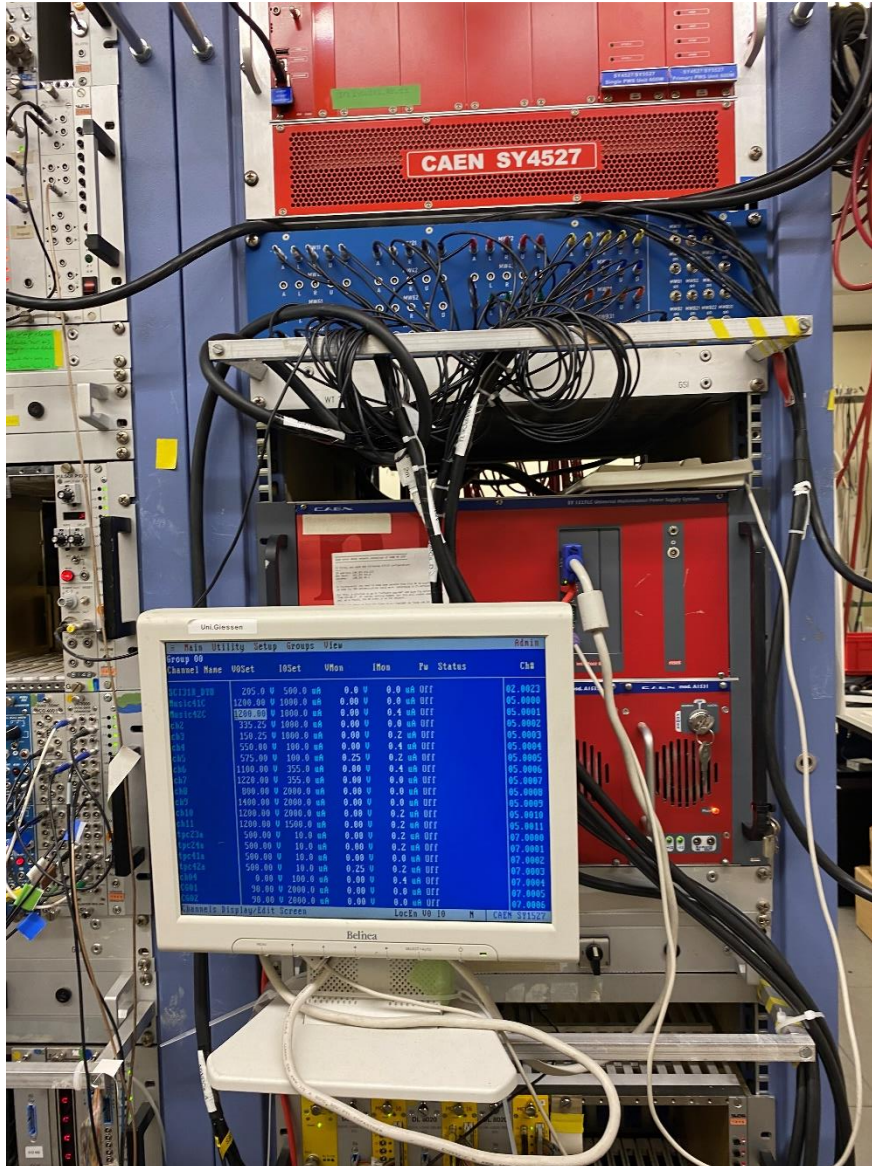
Figure 6: High voltage control (in massute) for MUSICs.
