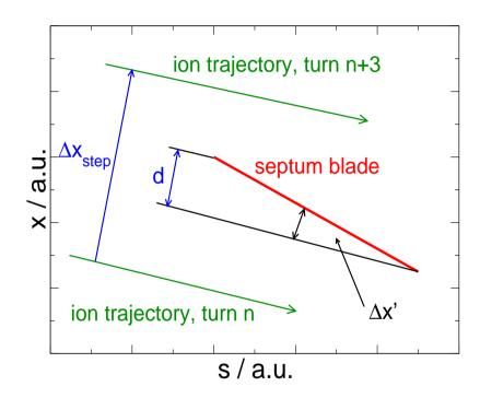
Inherent beam loss at septum blade due to particle collisions.
