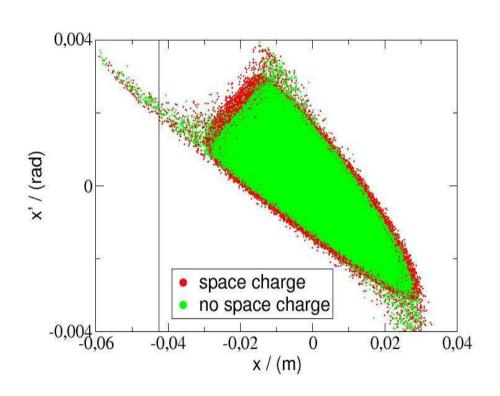
Formation of stable phase space area and separatrices also with magnet errors and/or space charge.
